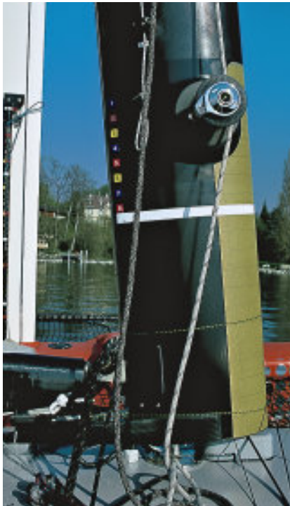
THE CARBON WINGMAST , which rotates as much as 45 degrees, is mounted on a ball on the central pod. In the background is one of the the boat's high-aspect daggerboards, which rides up and down on tracks, allowing it to be adjusted under load. Headsails are flown from the bowsprit, which is held true by a web of low-stretch line.
