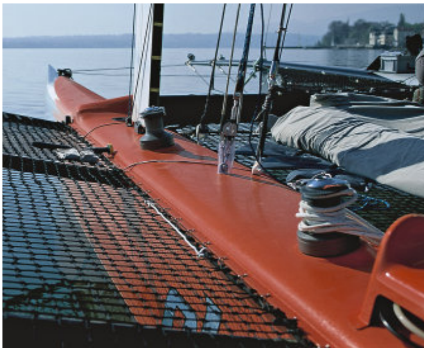
CAPSIZES ARE DISASTROUS , and expensive, so crew racks are required equipment. The helmsman's seat (right) is flanked by a hydraulic pump (not shown) used to trim the mainsheet.
